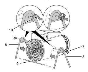
3. Secure the axle at the feet by means of the safety split pins (11).
