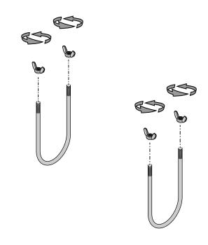
4. Position the respective U-bolt between either the first or the last two ribs at the device bottom.
