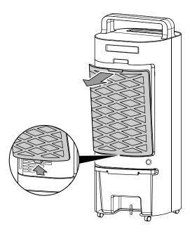
2. Remove the evaporation filter from the air filter.
